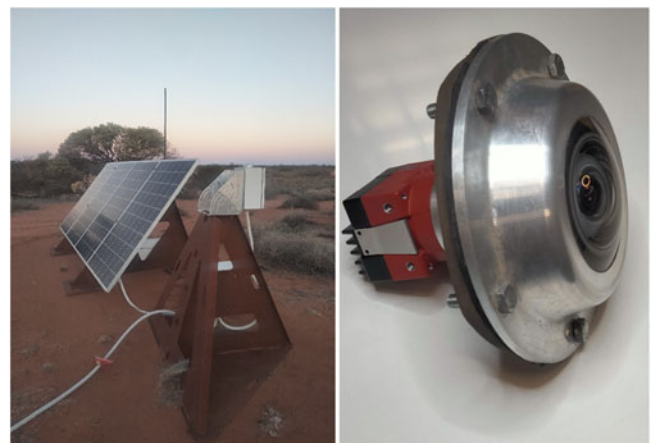
Figure 2. Left: Prototype installation near Perenjori, Western Australia. Right: Allied Vision Alvium U-052 USB machine vision camera connected to a weatherproofed Fujinon FE185C046HA lens assembly.
