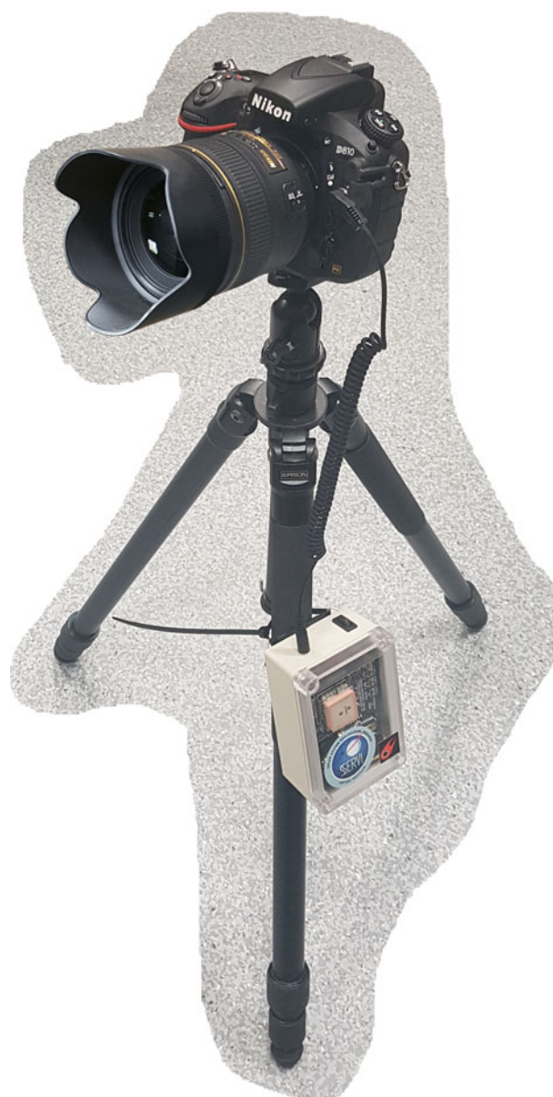
Figure 1. One of the observatories used in the OSIRIS-REx observation campaign, complete with the custom-designed triggering unit.
