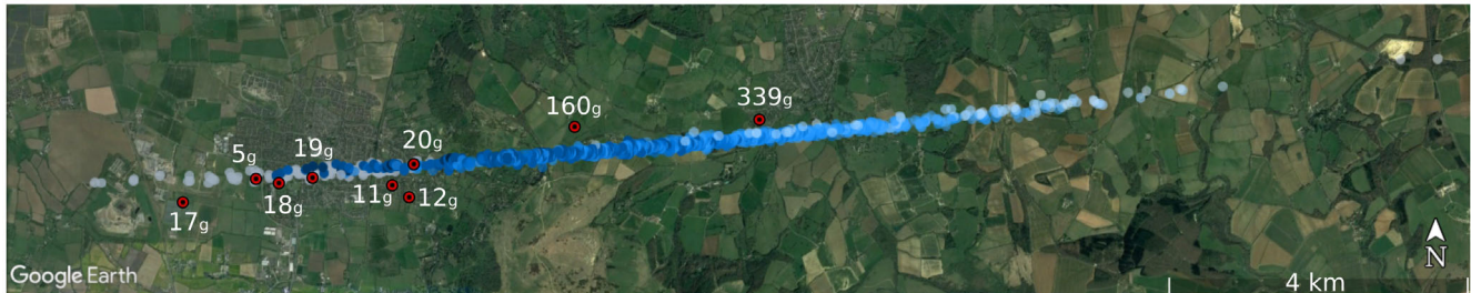
FIGURE 12. Fall line for the Winchcombe meteorite fall. Red points correspond to the location of the meteorites found with their estimated masses (Russell et al., 2022). Monte Carlo points from the darkflight simulation are blue shaded based on the assumed shape. In this case, the shape is the dominant parameter shifting the points along the fall line: dark blue are more brick-like and less aerodynamic in shape, while light blue is more sphere-like and aerodynamic shapes. Gray points to the west are from a custom model using an extreme, tile-like shape for reference.
