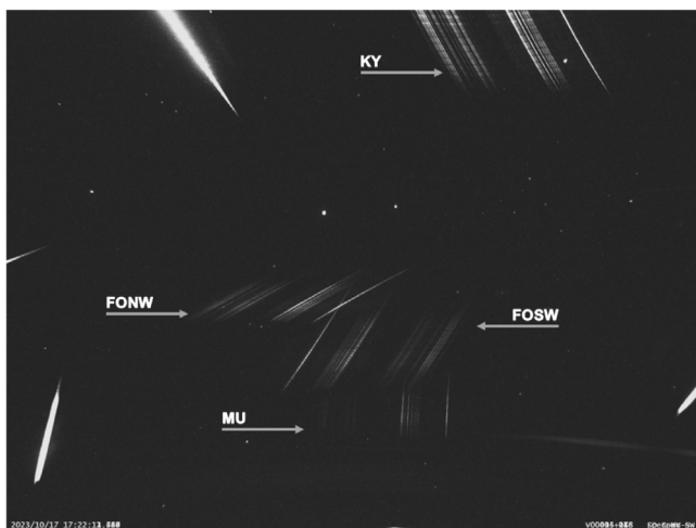
Fig. 4. Composite image displaying the spectrum of M20231017_172212 recorded by four AMOS spectrographs: Spec-MU, Spec-KY, Spec-FONW, and Spec-FOSW. The layout of these instruments is shown in Fig. 3.
