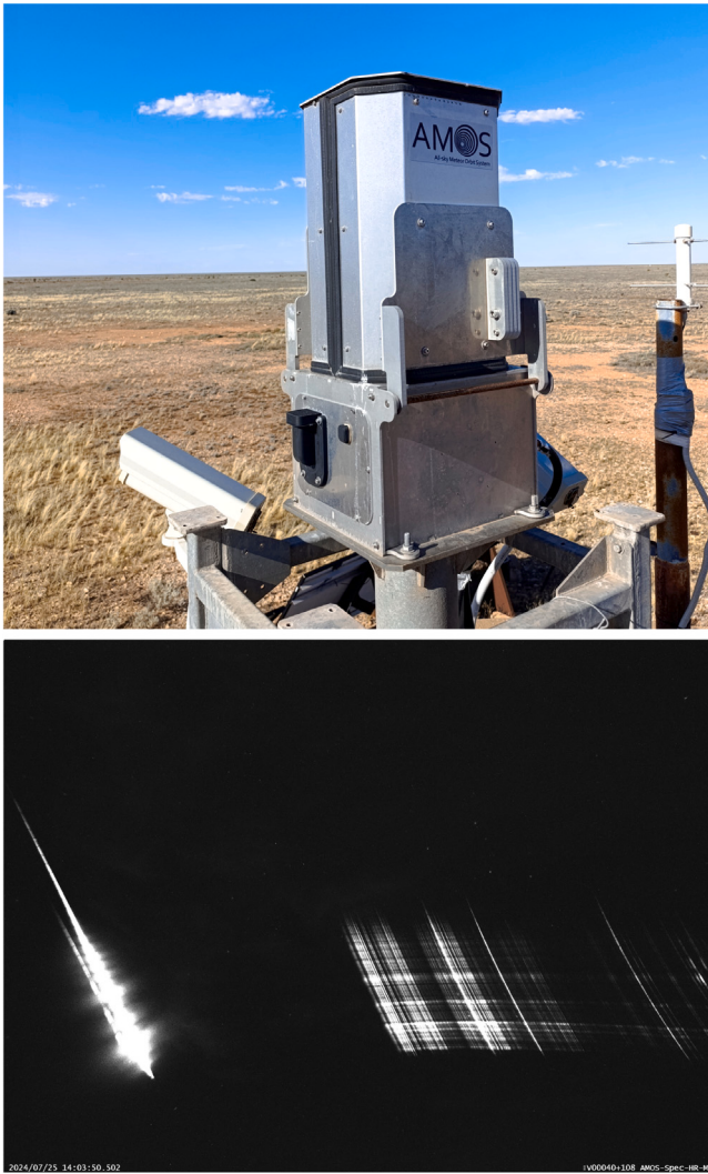
Fig. 2. Upper panel: typical configuration of the AMOS system, comprising the all-sky AMOS-Cam and the AMOS-Spec-HR spectrograph (shown in the lower left corner). Lower panel: composite image of meteor M20240725_140350 recorded by the AMOS-Spec-HR located on Mauna Kea, Hawaii.
