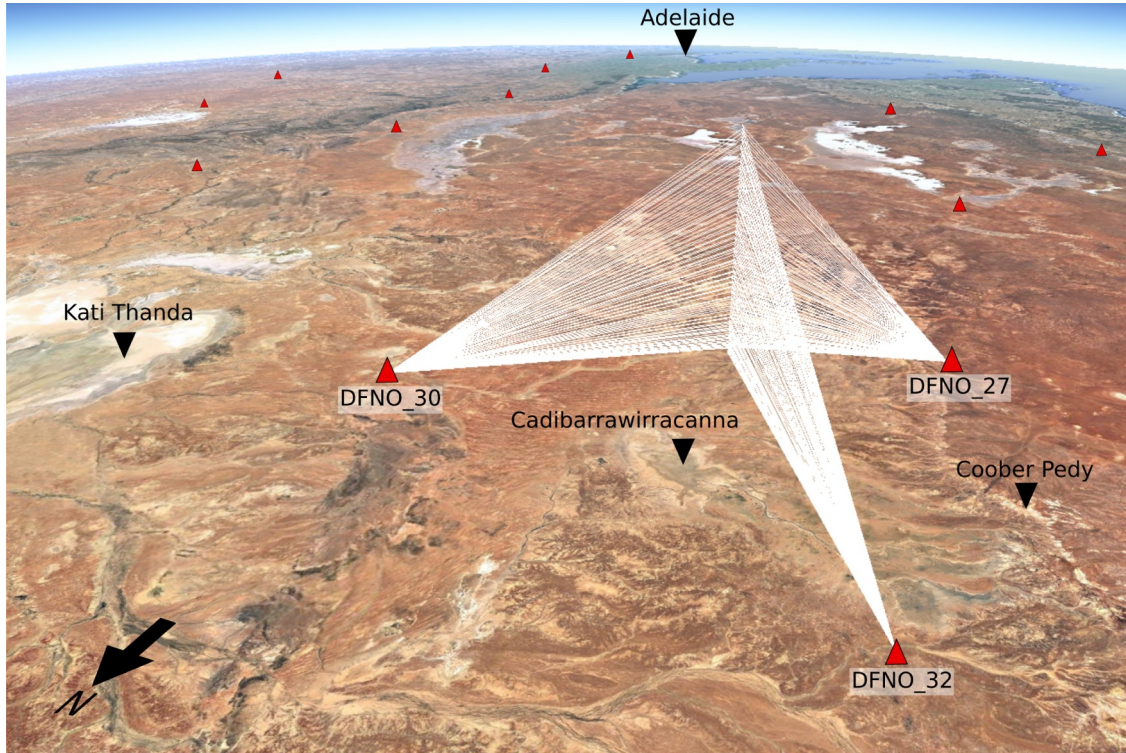
Fig. 8. Configuration of DN160410_03 observations. White observation rays correspond to the start and end points of the trajectory dashes in Fig. 7. (Google Earth image credit: Landsat/Copernicus).
