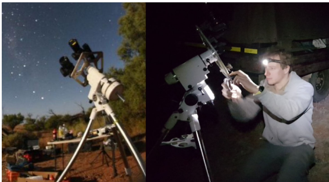
Fig. 5. Set up of spectral and tracking video on a manually operated mount (not in final position).
