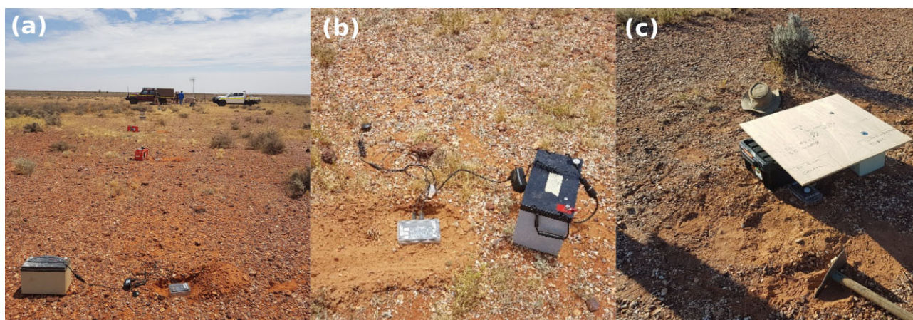
Fig. 6. (a), (b) Testing of Raspberry Shake sensors. (c) Sensors deployed in areas without bedrock were buried. (Color online)
