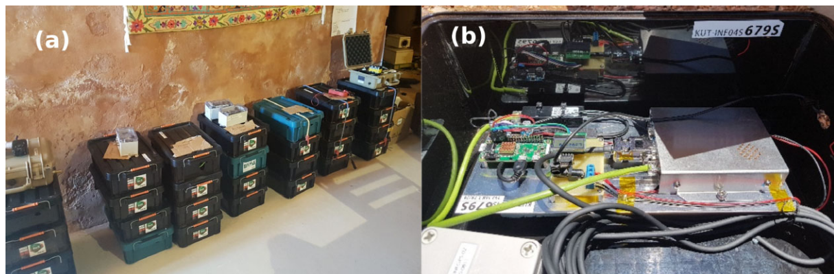
Fig. 7. (a) Seismo-acoustic instruments ready for deployment on December 3, including infrasound systems. (b) Interior setup of data logger, GPS and Raspberry Pi PC, Raspberry Shake instruments, and absolute barometers. (Color online)
