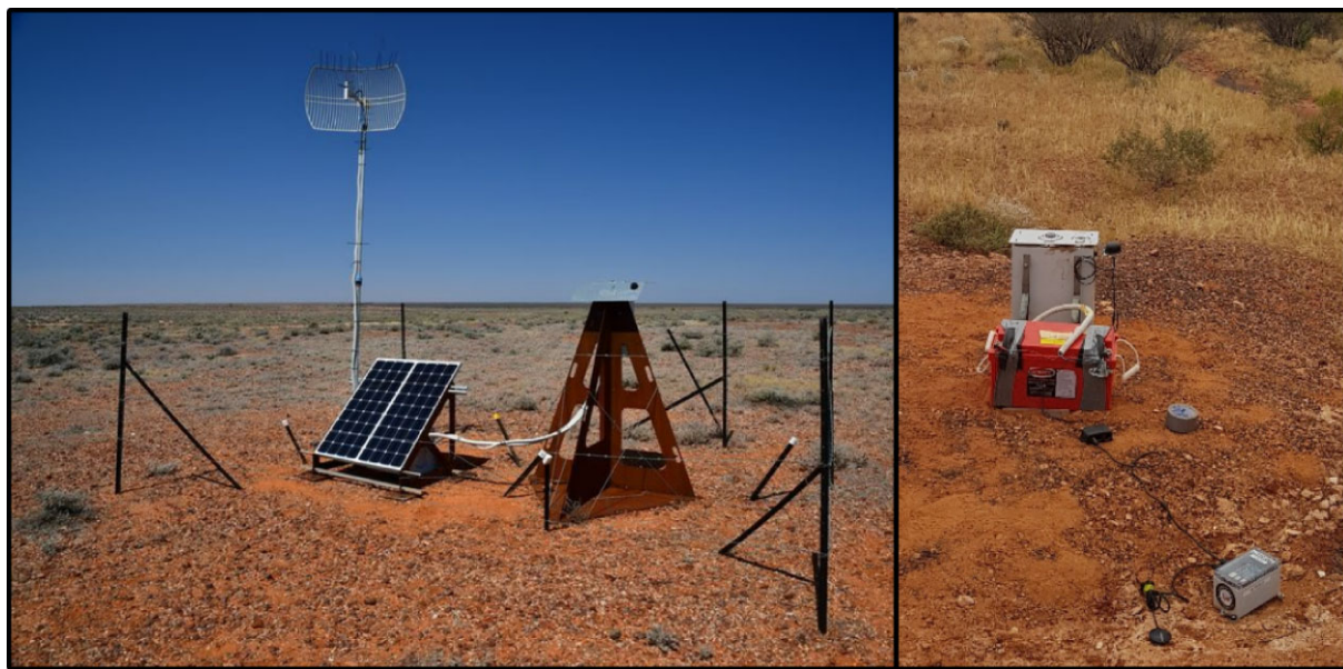
Fig. 4. Left: Permanent DFN observatory site at Ingomar (figure 3 site 3); Right: Temporary DFN camera setup at Jacob's Bore (figure 3 site 8), with 3D Raspberry Shake deployed on in situ bedrock. (Color online)
